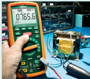
Measure the insulation resistance of transformer windings
