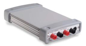
The U2741A USB DMM provides a broad range of essential features and 10 measurement functions: DC voltage and DC current; true-RMS AC voltage and AC current; two- and four-wire resistance; frequency; diode test; continuity; and temperature.
