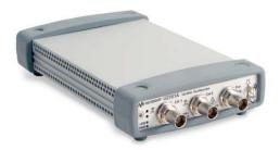
These USB scopes are available with bandwidths of either 100 MHz (U2701A) or 200 MHz (U2702A). Both provide 500 MSa/s sampling and 16 Mpts of memory per channel (1 GSa/s and 32 Mpts with two channels interleaved) to help you gain better insight into signal details. Advanced analysis capabilities built into the AMM scope software include waveform math and FFT with windowing. Other advanced features include:
