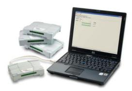
This group of three standalone units offers cost-effective DIO for applications such as driving relays, actuators and valves. Equipped with opto-isolation, they can also act as an interface to industrial sensors. Capabilities such as a failsafe watchdog timer and programmable power-up states ensure safe, predictable operation.
