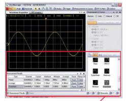
Simplify waveform analysis with automatic measurements such as 'rise time and duty cycle, and the measurement results panel.
