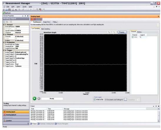
Monitor temperature measurements using the AMM interface.
