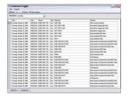
Capture and review configuration commands or convert the commands to snippets of VEE, VB, C++, and C# codes
