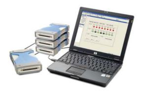
The three U2600A modules offer digital input and output with high channel count and opto-isolation. Virtual port grouping lets you select any eight input or output bits and group them into a single channel as a virtual DIO port. An interrupt function automatically triggers your system when a digital change of state occurs.
