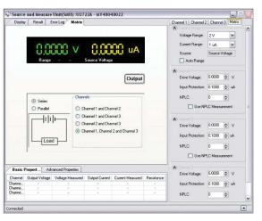
Combine channels for serial or parallel output.
