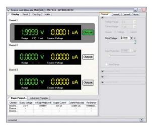
Configure all three channels separately to source or measure voltage or current.
