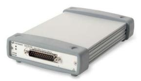
The U2751A is a high-quality, low-cost switching solution for complex testing. It has 32 two-wire crosspoints in a 4x8 configuration, enabling connection with any combination of rows and columns—including multiple channels at the same time. Other key features are 45-MHz bandwidth (without terminal block), a relay cycle counter, and a commandlogger function.
