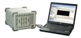
The U2781A is a six-slot chassis for Keysight USB modular instruments and data acquisition devices. It offers the convenience of one AC-power connection and a single USB link. Modules are hot-swappable and the auto-detection feature reduces setup time and effort. This 4U-high chassis also provides simultaneous synchronization between modules and enables SSI/star-trigger bus synchronization with an external trigger source.
