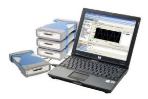
This family of three high-performance modules provides up to four channels per module with one analog-to-digital converter (ADC) for each channel. Maximum sampling rates are 2 MSa/s/ch in the U2531A (14 bits), 500 kSa/s/ch in the U2542A (16 bits) and 250 kSa/s/ch in the U2541A (16 bits).
