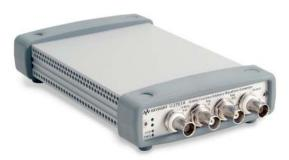
The U2761A USB function generator offers eleven standard signals as well as arbitrary waveforms. It relies on direct digital synthesis (DDS) to create stable, accurate output of low-distortion sine waves. The U2761A also provides square waves with fast rise and fall times up to 20 MHz and linear ramps up to 200 kHz. For simulation of real-world signals, use the waveform editor to create arbitrary waveforms with 14-bit resolution up to 200 kHz.
