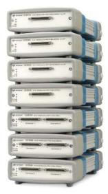
This high-performance series consists of four basic models and three high-density models. The basic models feature 16 single-ended/eight differential inputs with 16-bit resolution and ±10 V maximum range. The high-density models offer 64 single-ended/32 differential inputs with 16-bit resolution in the lower-speed models and the 12-bit resolution in high-speed U2331A.
