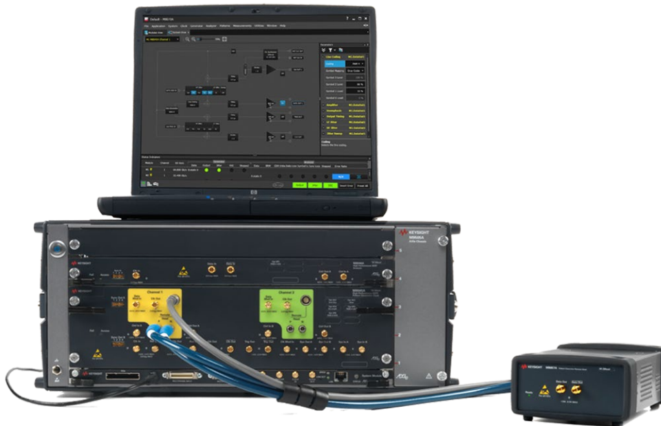
M8040 64 GBaud high-performance BERT, M9537A embedded controller in a M9505A 5-slot AXIe chassis.
