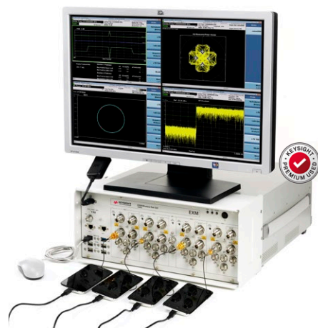
The EXM wireless test set can test up to 4 devices at the same time.
