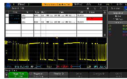
Figure 17. CAN-FD decode and trigger.
