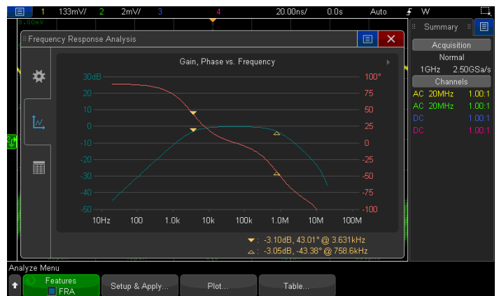
Figure 25. Frequency response analysis plot (Bode gain & phase) of a bandpass filter.
