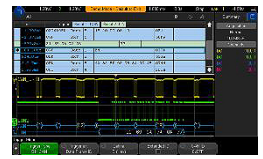
Figure 19. Multi-bus time aligned decode.
